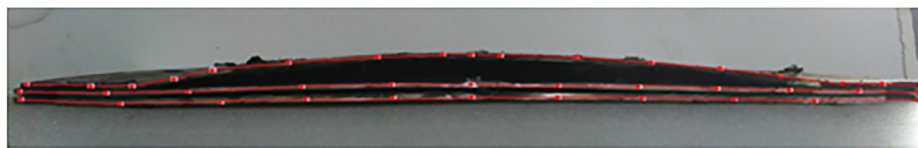
图8 敷设泡沫覆盖层的钢板与未敷设的钢板变形 Fig. 8 The steel plate deformation with foam coating and without coating
