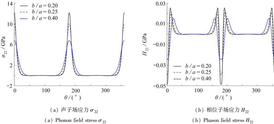
图6 取  $a = 0.2$  m, 孔边应力值随  $b$  的变化情况Fig. 6 For  $a = 0.2$  m, the changes of hole edge stresses with  $b$
