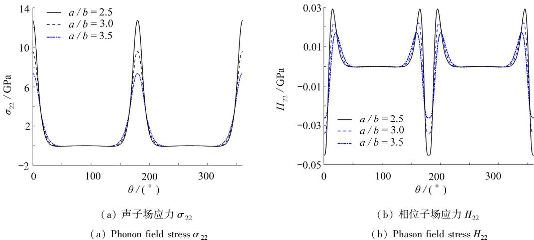
图7 取  $b = 0.1$  m, 孔边应力值随  $a$  的变化情况Fig. 7 For  $b = 0.1$  m, the changes of hole edge stresses with  $a$
