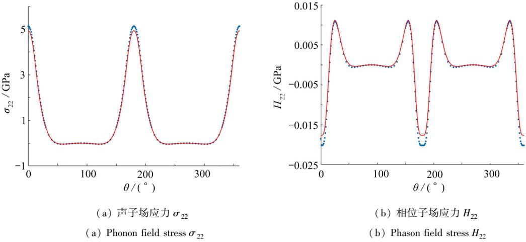
图5 边界元解与无限大板解析解对比 ( $H/a = 40, W/a = 8$ )Fig. 5 Comparison of the boundary element solution and the infinite plate analytical solution ( $H/a = 40, W/a = 8$ )
