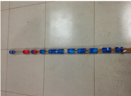
图 5 贴完应变片的管道 Fig.5 The pipeline with strain gages
